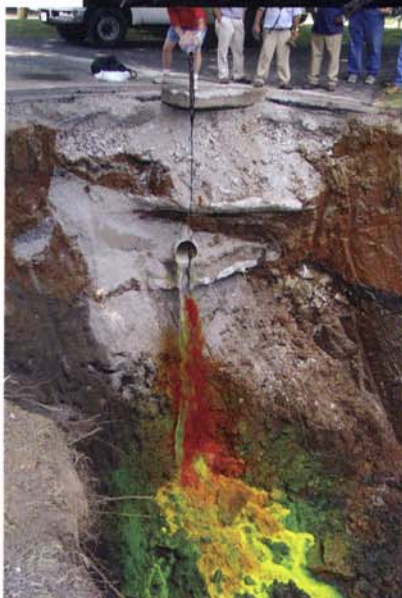
Use of fluorescent dye to trace ground water flow
